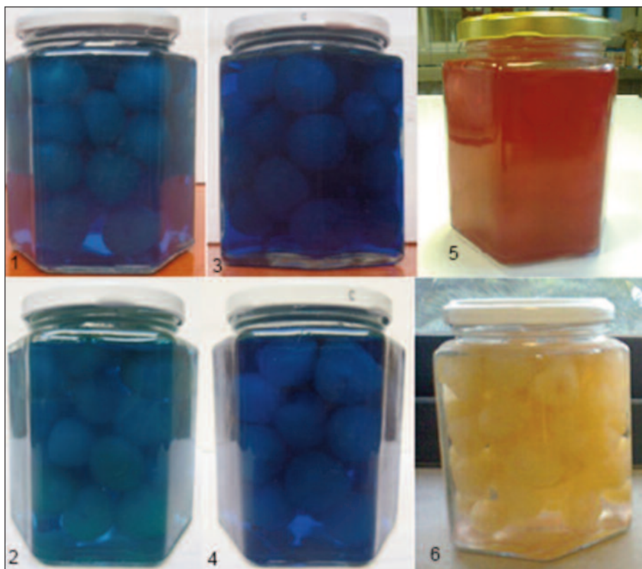
1- T3 Light Blue Brillant before life test. 2- T3 Light Blue Brillant after life test. 3- T2Dark Blue Brillant before life test. 4- T2Dark Blue Brillant after life test. 5- T1 ErB before life test. 6- T1ErB after life test.
